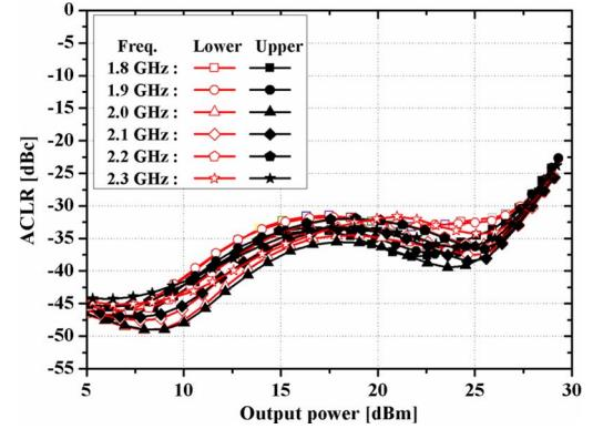
Fig. 10. ACLR measurement results from 1.8 to 2.3 GHz.
