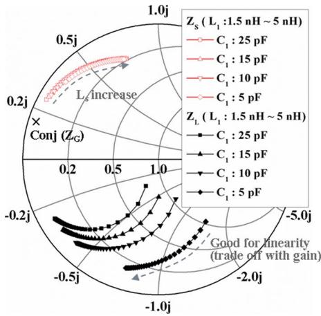
Fig. 5. Load impedance ( $Z_L$ ) of the driver amplifier and source impedance ( $Z_S$ ) to ensure that the maximum linear power exceeds 28 dBm at an  $IMD_3$  level of  $-25$  dBc at 1.95 GHz.
