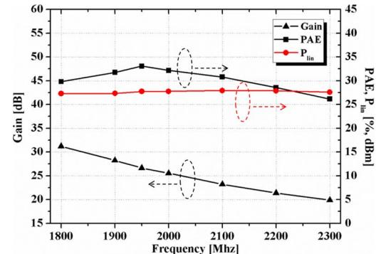
Fig. 11. Measured linear output power at an ACLR<sub>E-UTRA</sub> of  $-30 \text{ dBc}$ , with the gain and efficiency from 1.8 to 2.3 GHz.
