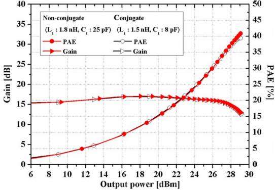
Fig. 4. Gain and PAE achieved by a two-tone simulation at 1.95 GHz. The results show two cases of conjugate matching and nonconjugate matching at  $Z_s$ .
