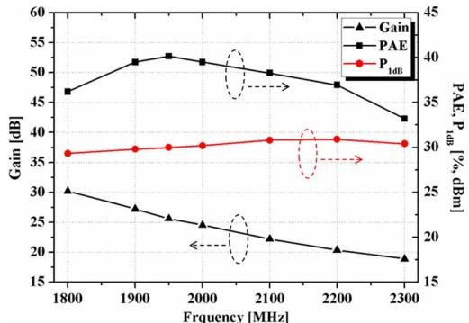
Fig. 9. CW measurement results from 1.8 to 2.3 GHz at a 1-dB compression point.
