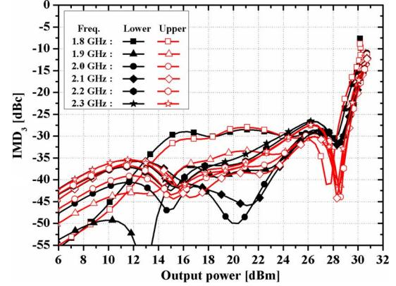
Fig. 6. Two-tone  $IMD_3$  simulation results from 1.8 to 2.3 GHz, when the linear matching points in Fig. 5 are applied at interstage matching.
