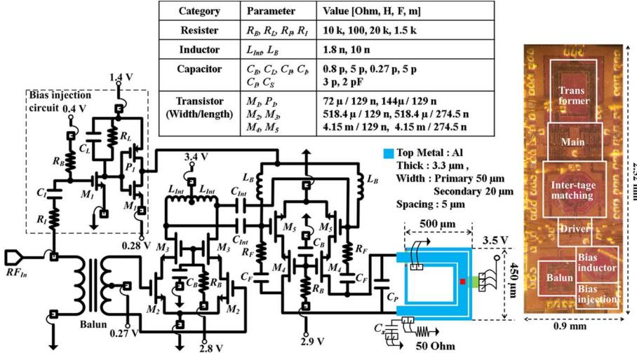
Fig. 7. Schematic of the two-stage fully integrated broadband linear CMOS PA. The geometry of the transformer and a chip photograph are also shown.
