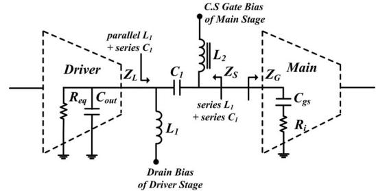
Fig. 1. Interstage matching network for broadband linear output power.
