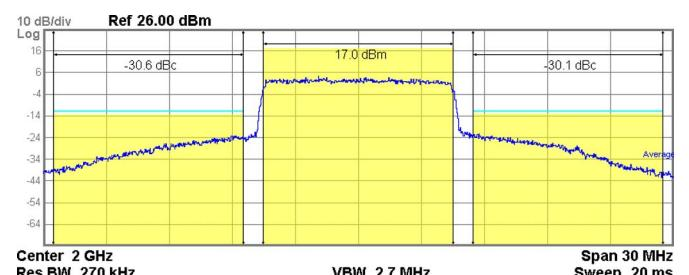
Fig. 12. Output spectrum with 27.76 dBm at 2 GHz.
