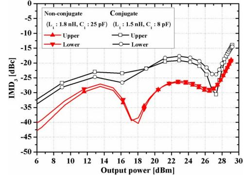
Fig. 3. Two-tone  $\text{IMD}_3$  simulation results at 1.95 GHz. The results show two cases of conjugate matching and nonconjugate matching at  $Z_s$ .
