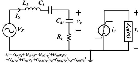
Fig. 2. Thevenin-equivalent circuit at  $Z_s$  in Fig. 1.
