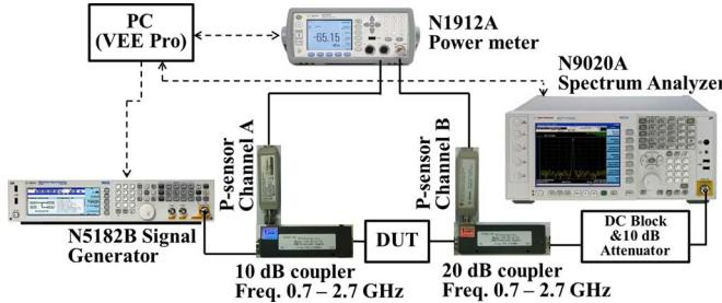
Fig. 8. Measurement setting for the designed PA (DUT) test.
