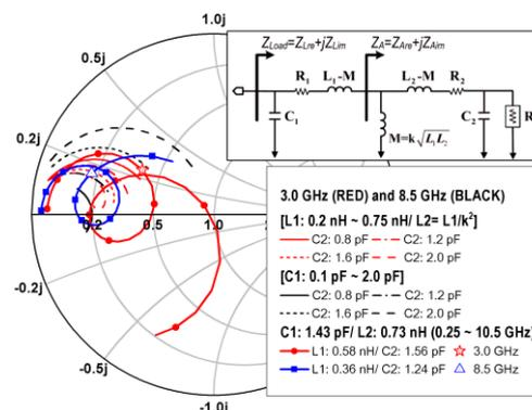
Fig. 1. Normalized  $Z_{\text{Load}}$  with variations of  $L_1$ ,  $L_2$ ,  $C_1$ , and  $C_2$  at the S/X-band.
