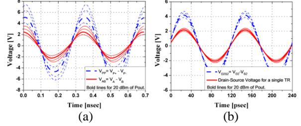
Fig. 5. Simulated voltage difference waveforms: (a) A and B nodes and P+ and P- nodes for S-band operation, and (b)  $D_2$  and  $S_2$  nodes and drain-to-source of a single transistor.
