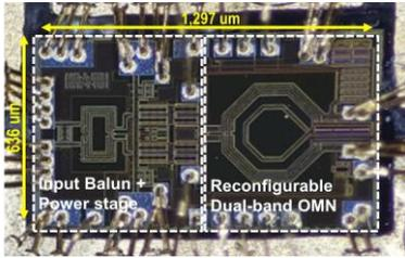
Fig. 7. Microphotograph of PA testing module.
