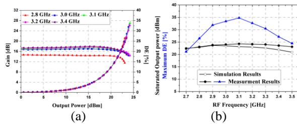
Fig. 8. Measured gain and DE as a function of output power with CW sources in (a) the S-band and (b) the X-band.
