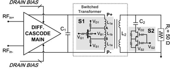
Fig. 2. Schematic of reconfigurable dual-band output matching network with single PA.
