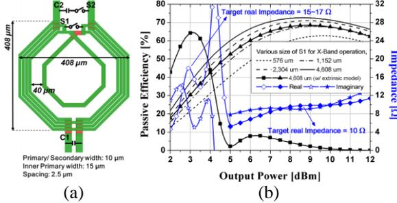
Fig. 3. (a) Physical layout of the OMN, (b) Passive efficiencies with various sizes of S1 and complex impedances for the S/X-band operation.
