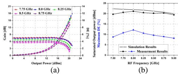
Fig. 9. Measured P<sub>SAT</sub> and DE versus frequencies in (a) the S-band and (b) the X-band.
