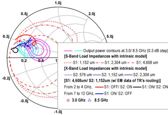
Fig. 4. Normalized  $Z_{Load}$  according to various sizes of S1/S2 and different switch operations.
