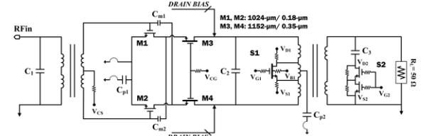
Fig. 6. Schematic of reconfigurable dual-band CMOS PA.
