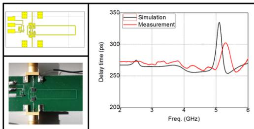
Fig. 5. CST model, fabrication model and simulation & measurement results of conventional switched line with 2 switches (Delay time difference: 270ps).
