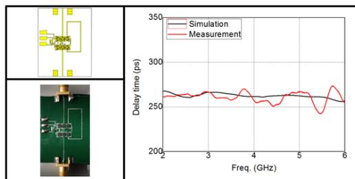
Fig. 6. CST model, fabrication model and simulation & measurement results of proposed switched line using cascaded switches with 6 switches (Delay time difference: 270ps).
