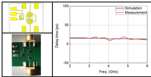
Fig. 4. CST model, fabrication model and simulation & measurement results of conventional switched line with 2 switches (Delay time difference: 15ps).
