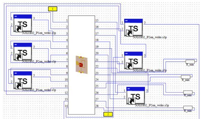
Fig. 3. Block diagram of proposed switched line using cascaded switches (CST design studio).
