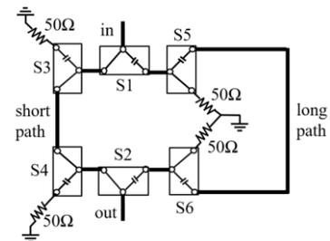
Fig. 2. Proposed switched line using cascaded switches.
