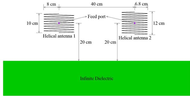
Fig. 11. Simulation configuration for Section VII-B.
