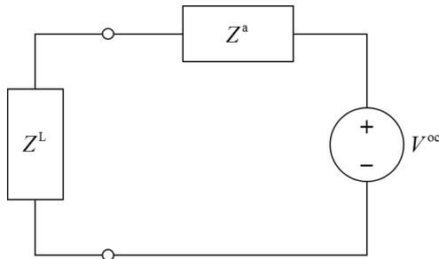
Fig. 3. Equivalent circuit for a receiving antenna.
