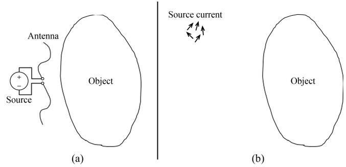
Fig. 4. Method for calculating the open-circuit voltage of equivalent circuit for a receiving antenna in the scenario in Fig. 2. (a) Situation in which the input impedance  $Z^a$  and electric current density  $\mathbf{J}^{at}$  of an antenna in transmitting mode is determined. (b) Situation in which the electric field  $\mathbf{E}^{in}$  is determined.
