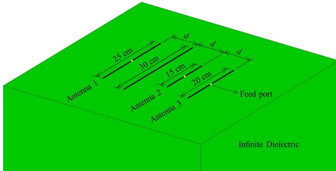
Fig. 8. Simulation configuration for Section VII-A.
