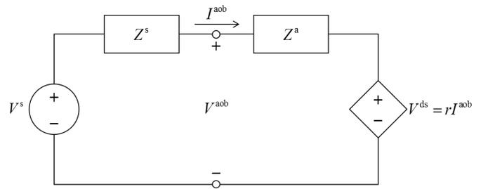
Fig. 5. Equivalent circuit for a transmitting antenna with type A and type B objects.
