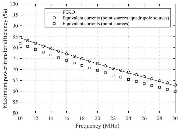
Fig. 14. Maximum power transfer efficiency between helical antennas in half-space.
