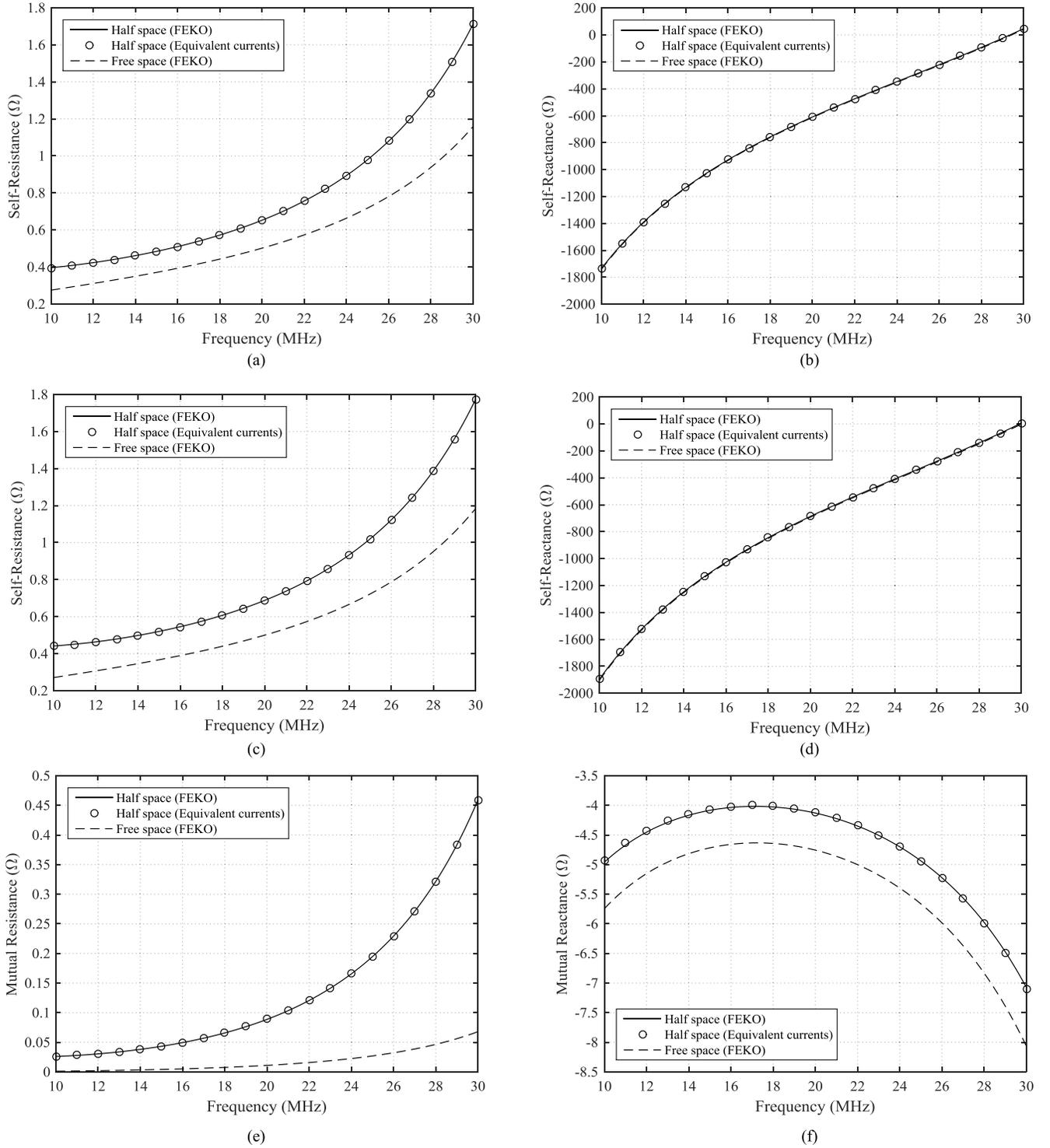
Fig. 13. Impedance parameters of helical antennas in half-space and free space. (a) Real part of  $Z_{11}$ . (b) Imaginary part of  $Z_{11}$ . (c) Real part of  $Z_{22}$ . (d) Imaginary part of  $Z_{22}$ . (e) Real parts of  $Z_{21}$  and  $Z_{12}$ . (f) Imaginary parts of  $Z_{21}$  and  $Z_{12}$ .
