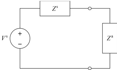
Fig. 1. Equivalent circuit for a transmitting antenna.
