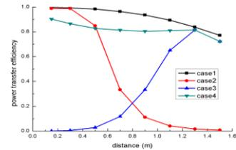
Fig. 3. Comparison of the power transfer efficiency for two coupled small spiral antennas (case 1: fixed frequency with simultaneous matching condition; case 2: frequency tracking with 50 ohm load impedance; case 3: fixed frequency with fixed load impedance (optimum impedance at 1.5 m); case 4: frequency tracking with fixed load impedance (optimum impedance at 1.5 m))
