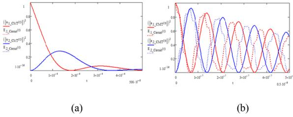
Fig. 8. Normalized energy flows analyzed by Coupled-mode theory and transient circuit theory in each resonator as function of time: (a) Weak-coupling, High-Q, (b) Strong-coupling, Low-Q
