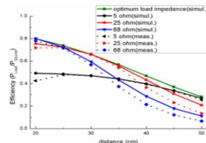
Fig. 4. The total power transfer efficiency for two coupled antennas (line: simulated results including the balun loss and assuming that PA efficiency is 100%, dot: the efficiencies are measured results)
