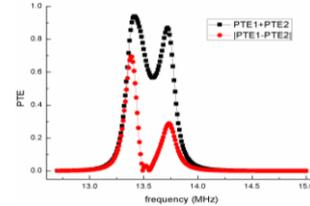
Fig. 6. The maximum power transfer efficiencies of antennas with different radiation efficiencies
