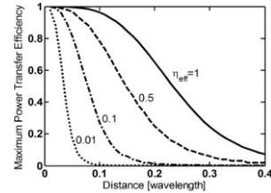
Fig. 1. The maximum power transfer efficiencies of antennas with different radiation efficiencies
