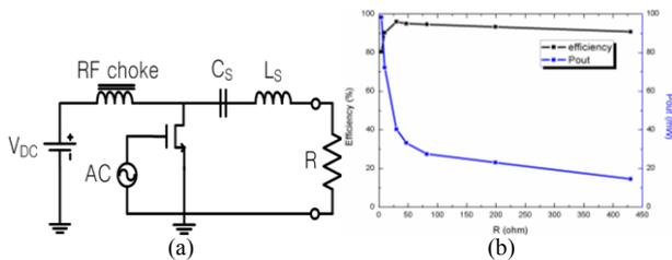
Fig. 2. The schematic, efficiency and output power of PAs against the load resistance: (a) schematic of Class-D PA ( $V_{DC}=1V$ ,  $C_S=58pF$ ,  $L_S=15uH$ ), (b) efficiency and output power
