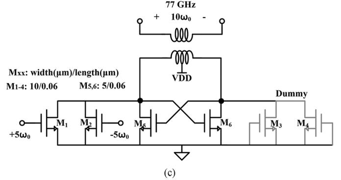
Fig. 9. Schematic of ×10 frequency multiplier. (a) STD circuitry and ring OSC. (b) Five-push frequency adder. (c) Push-push frequency doubler.
