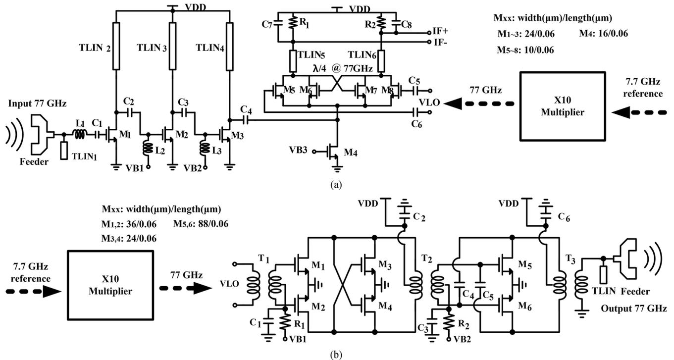
Fig. 10. Frequency multiplier based Tx and Rx with on-chip feeders. (a) Rx with an on-chip feeder. (b) Tx with an on-chip feeder.
