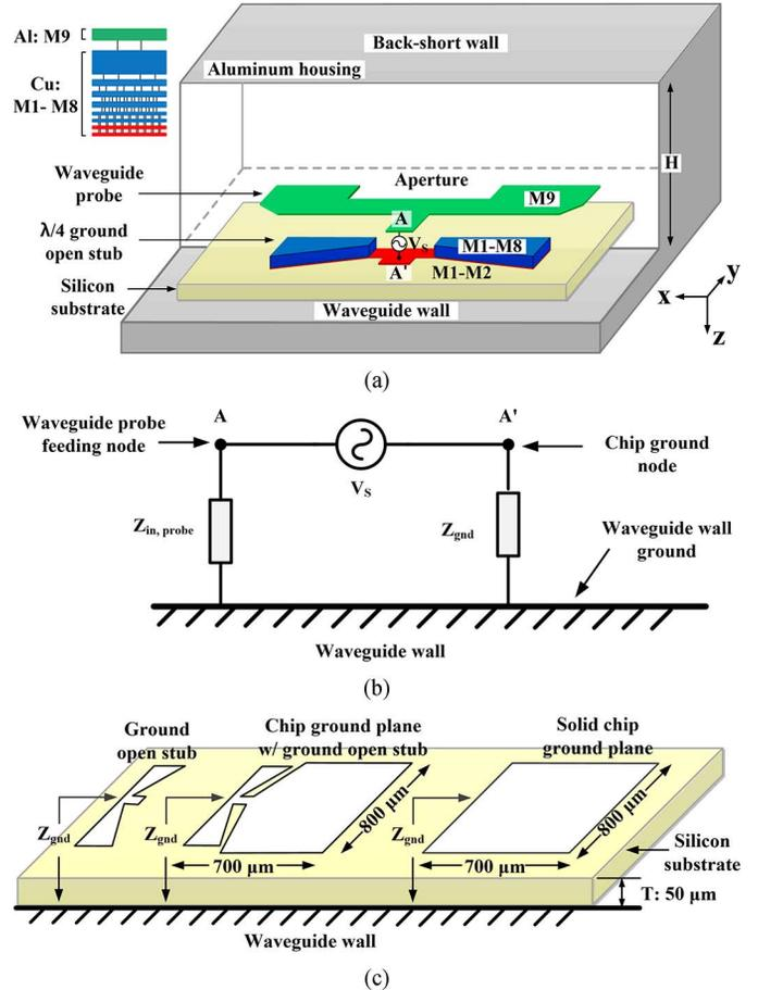
Fig. 2. Proposed on-chip waveguide feeder. (a) 3-D view and metal layers. (b) Electrical equivalent circuit of the proposed waveguide feeder. (c) Three simulation structures to compare the impedance  $Z_{\text{gnd}}$ .
