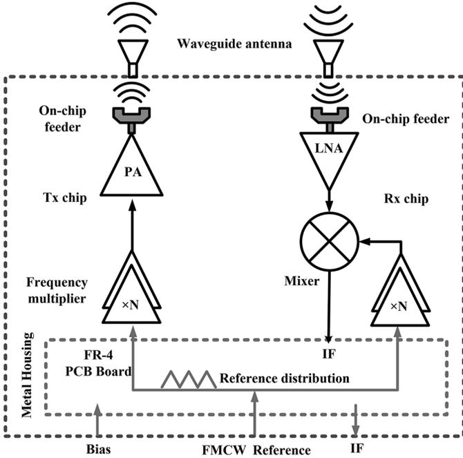
Fig. 1. Proposed FMCW radar architecture.
