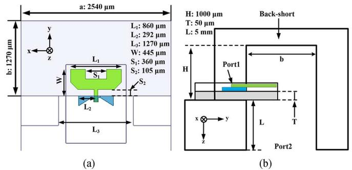
Fig. 4. Proposed on-chip waveguide feeder. (a) Top view in  $xy$ -plane. (b) Side view in  $yz$ -plane.
