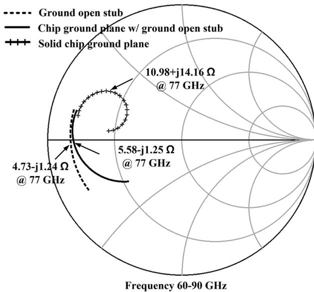
Fig. 3. Simulation results of  $Z_{\text{gnd}}$  between chip ground node and waveguide wall ground.
