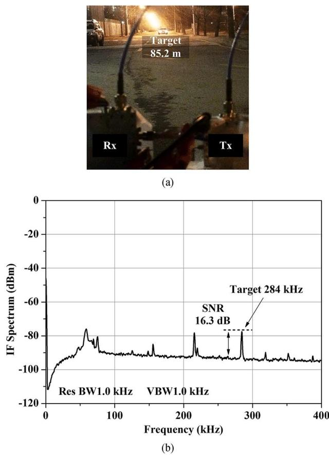
Fig. 19. Outdoor range detection measurement results. (a) Experiment environment. (b) Measured IF spectrum with the target 85 m away.
