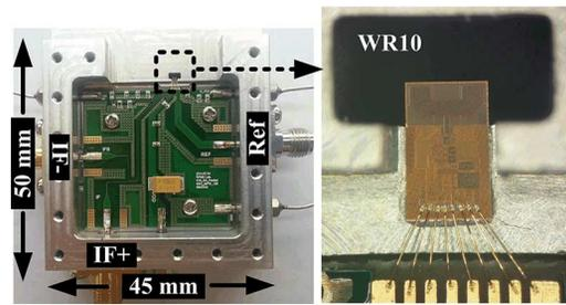
Fig. 16. Fabricated Rx module with an on-chip feeder mounted on the aperture.
