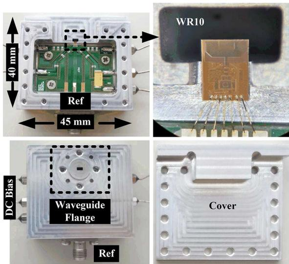
Fig. 14. Fabricated Tx module with an on-chip feeder mounted on the aperture.
