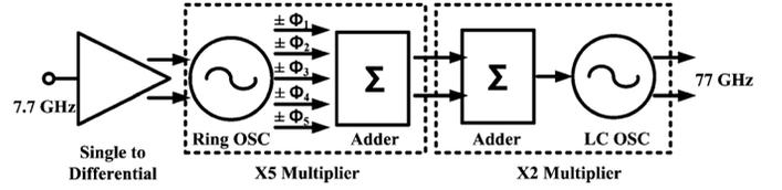
Fig. 8. Block diagram of ×10 frequency multiplier.
