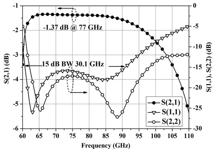
Fig. 5. S-parameter simulation results of the on-chip waveguide feeder using 3-D EM simulator.
