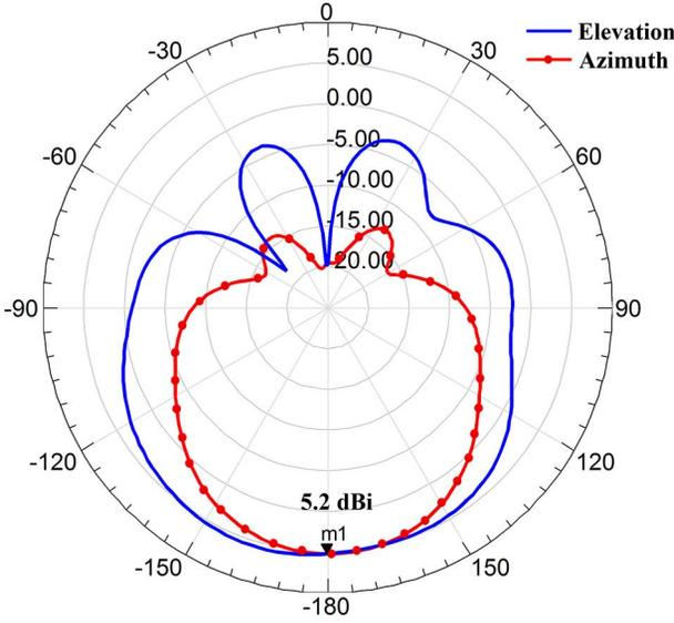
Fig. 7. Simulation results of radiation patterns of WR10 aperture fed by the proposed on-chip feeder. The length of the waveguide is 1 mm. Elevation pattern (*E*-plane), azimuthal pattern (*H*-plane).
