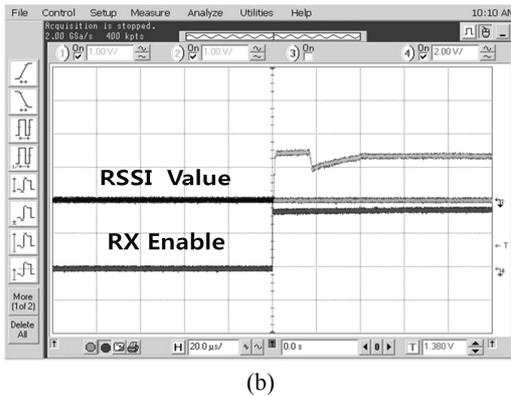
**Fig. 10.** Measured RSSI : (a) transfer curve, (b) transient response.
