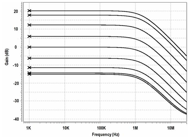
**Fig. 5.** AC simulation result of the proposed VGA.
