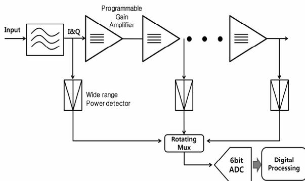
Fig. 1. Block diagram of the proposed RSSI architecture.
