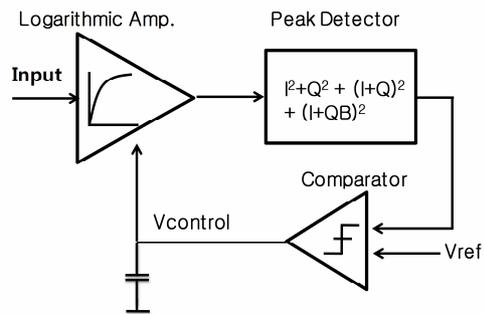
Fig. 3. Structure of the wide range power detector.
