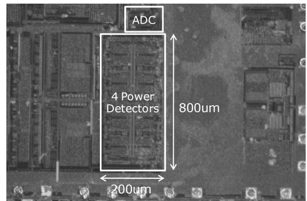
**Fig. 8.** Chip microphotograph.
