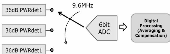
Fig. 2. Shared ADC for 3 power detectors.
