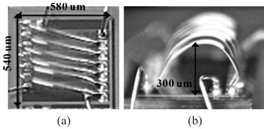
Fig. 2 Chip photograph of the transformer. (a) Top view. (b) Side view.
