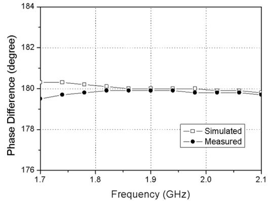
Fig. 5 Frequency response of differential phase output at the secondary.
