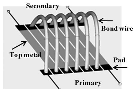
Fig. 1 Perspective view of a proposed transformer using bond wires.
