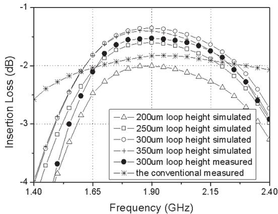
Fig. 4 Simulation and measurement of insertion loss of the proposed and the conventional transformers.
