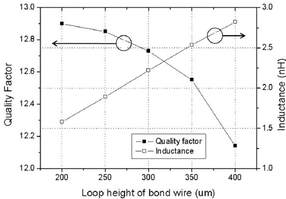
Fig. 3 Simulated Q factor and inductance versus the loop height.
