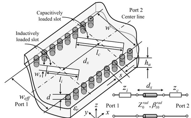
Fig. 1. The alternating reactance slot pair etched on the broad wall of a radiating SIW and its equivalent circuit, where  $Z_0^{\text{rad}}$  is the wave impedance and  $\beta_{10}^{\text{rad}}$  is the propagation constant of the TE<sub>10</sub> mode [3].
