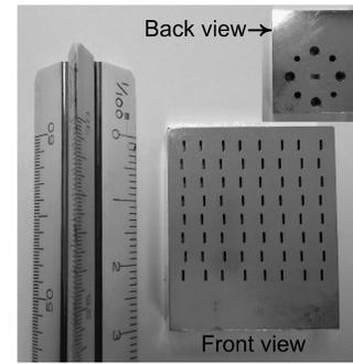
Fig. 4. The fabricated W-band 8 by 8 slot array antenna using electroforming technique [2].
