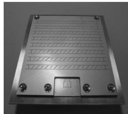
Fig. 3. The fabricated planar slot array antenna for Ka-Band [3].
