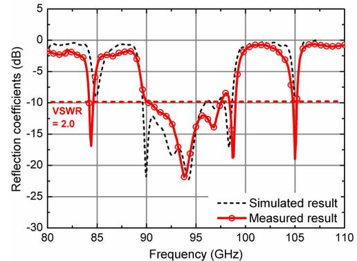
Fig. 5. The reflection coefficient [2].
