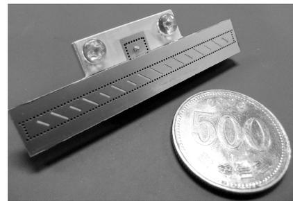
Fig. 2. The fabricated linear slot array antenna for Ka-Band [4].
