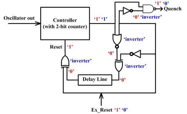
Fig. 6. The digital block for self-quench.
