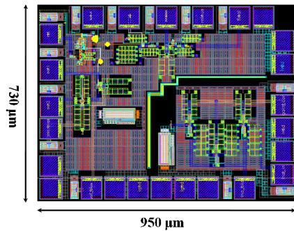
Fig. 8. The designed receiver chip layout
