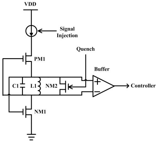
Fig. 5. LC-Oscillator circuit with buffer
