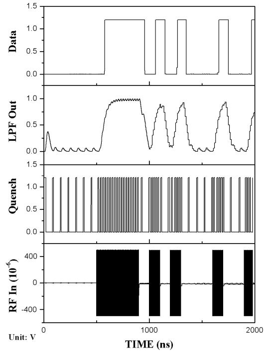
Fig. 9. The transient simulation of proposed receiver.
