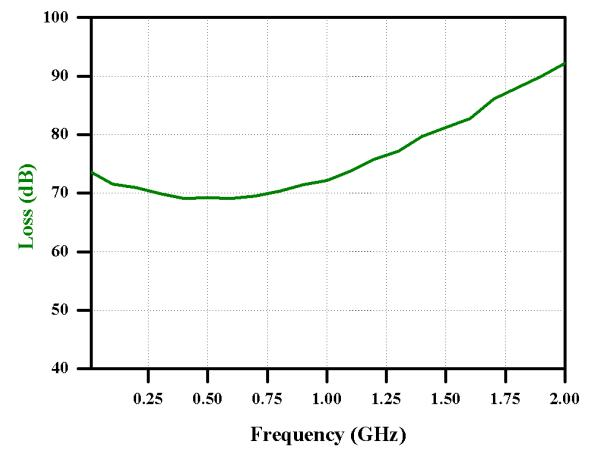
Fig. 3. The propagation loss in human body.
