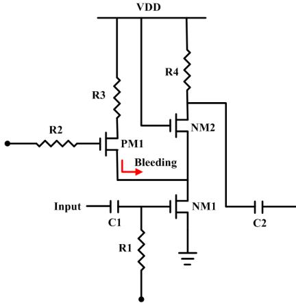
Fig. 4. Isolation amplifier circuit
