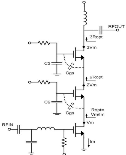
Figure 1. Schematic of conventional triple stacked PA
