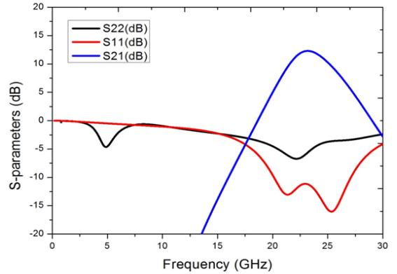
Figure 4. Simulated S-parameters of triple stacked PA
