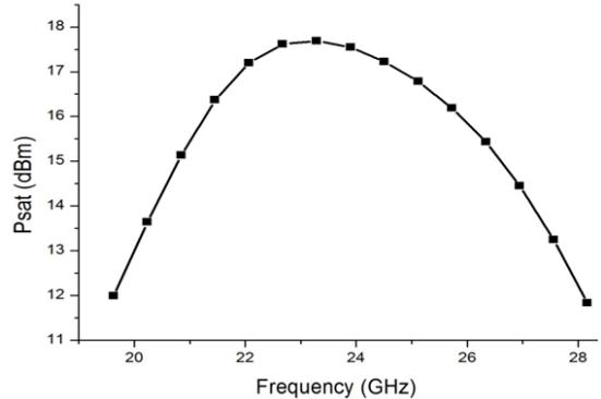
Figure 6. Simulated saturated ouput power (Psat) as a function of frequency
