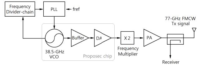
Figure 1. A concept of 77-GHz FMCW radar transmitter.
