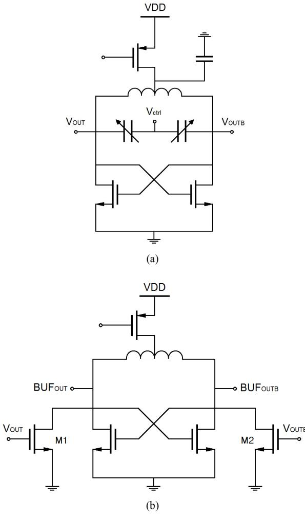
Figure 3. (a) VCO schematic. (b) Injection-locking buffer schematic.
