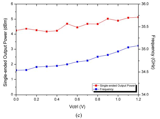
Figure 2. (a) Chip micro-photograph. (b) Phase noise. (c) Single-ended output power and output frequency vs. control voltage.
