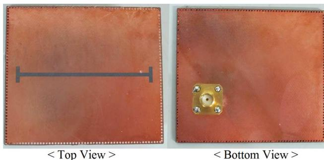
Fig. 4. Fabricated wideband cavity-backed slot antenna.
