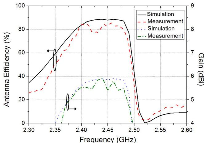
Fig. 6. Comparison of measured and simulated total efficiency and antenna gain of the proposed antenna.
