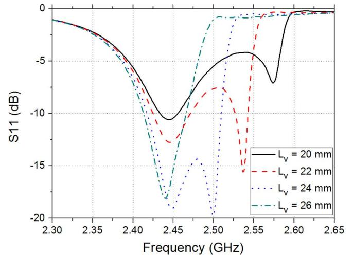
Fig. 3. Effect of via location on the reflection coefficient. All other parameters are kept as described in Fig. 1.
