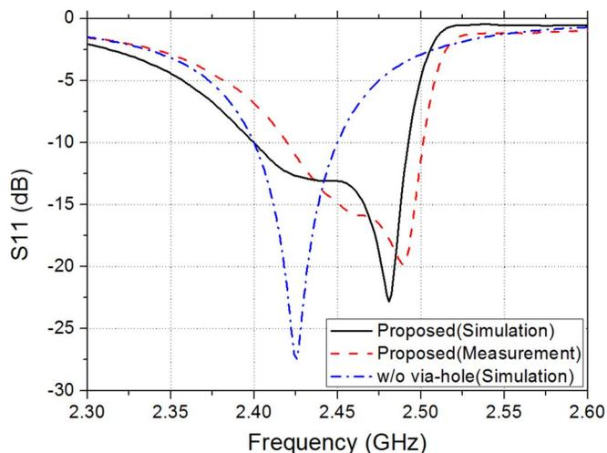
Fig. 5. Comparison of the reflection coefficient of the proposed antenna and a conventional cavity-backed slot antenna without via-hole.
