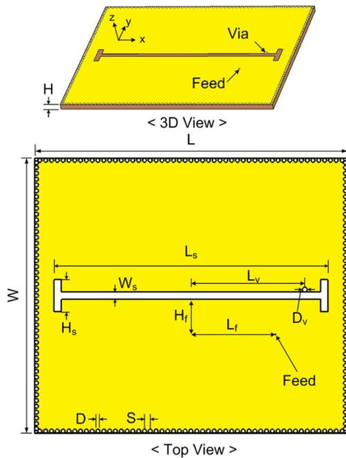
Fig. 1. Structure of wideband cavity-backed slot antenna. ( $W = 55.8$ ,  $L = 63.8$ ,  $H = 1.57$ ,  $L_s = 55.75$ ,  $H_s = 6.6$ ,  $W_s = 1.5$ ,  $L_v = 23.5$ ,  $D_v = 1$ ,  $H_f = 7.25$ ,  $L_f = 17.5$ ,  $D = 0.8$ ,  $S = 1.2$ , all in the unit of millimeters).
