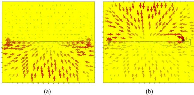
Fig. 2. Current distribution of proposed structure at each resonance. (a) At first resonance and (b) at higher frequency when second resonance occurs.
