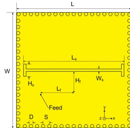
Fig. 1. Geometry of simulated and measured cavity-backed slot antenna. (Dimensions of the fabricated antenna,  $W = 45$ ,  $L = 55$ ,  $L_s = 41$ ,  $H_s = 1$ ,  $W_s = 1$ ,  $H_f = 9.5$ ,  $L_f = 13$ ,  $D = 0.7$ ,  $S = 2.5$ , all in the unit of millimeters.)
