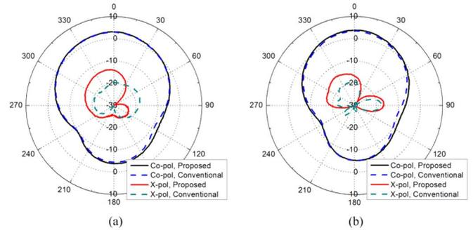
Fig. 9. Measured radiation patterns of the proposed and conventional cavity-backed slot antenna. (a) E-plane ( $yz$ -plane) (b) H-plane ( $xz$ -plane).
