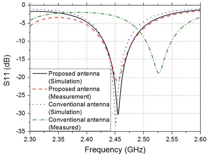
Fig. 7. Reflection coefficient of simulated and measured antenna.
