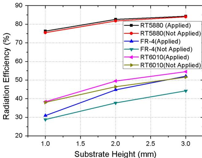
Fig. 4. Simulated radiation efficiency of the cavity-backed slot antenna on different substrates.
