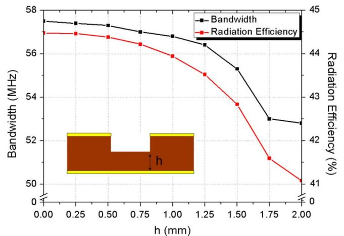
Fig. 5. Simulated  $-10$ -dB bandwidth with variations of removing depth.
