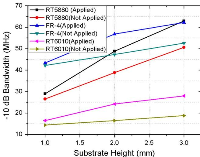
Fig. 3. Simulated  $-10$ -dB bandwidth of the cavity-backed slot antenna on different substrates.
