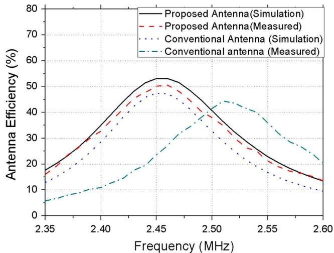
Fig. 8. Simulated and measured antenna efficiency.
