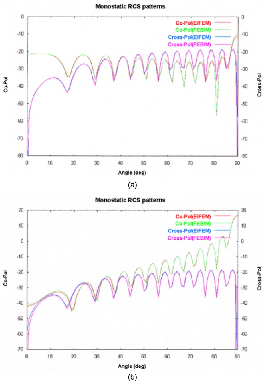
Fig. 3 Monostatic RCS patterns of a 3D long crack recessed in the ground plane (  $a=10\lambda$ ,  $b=0.1\lambda$ ,  $c=0.1\lambda$ ,  $\theta=40^\circ$  )
