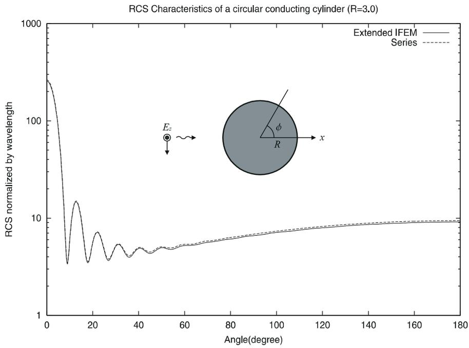
Fig. 2 (a) Surface current density and (b) bistatic RCS patterns when  $R = 3.0\lambda$
