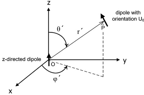
Fig. 1. Two coupled dipoles with arbitrary orientation [10].
