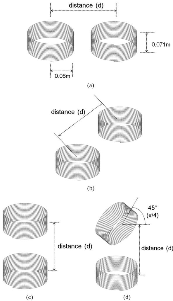
Fig. 2. Two coupled small helix antennas: (a) parallel configuration, (b) diagonal configuration, (c) collinear configuration, and (d)  $\pi/4$ -tilted collinear configuration.
