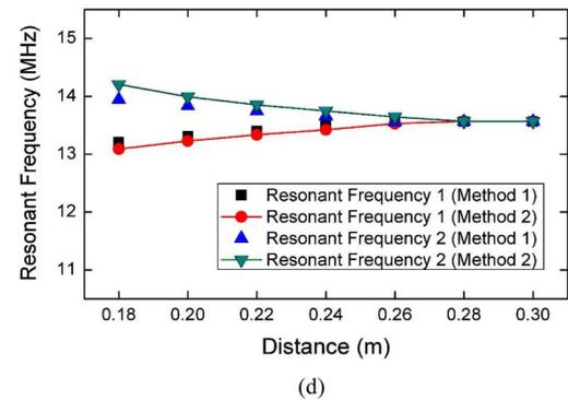
Fig. 3. Comparison of the resonant frequencies for two coupled small helix antennas: (a) parallel configuration, (b) diagonal configuration, (c) collinear configuration, and (d)  $\pi/4$ -tilted collinear configuration. (Method 1: the full EM simulation; Method 2: the proposed method based on the addition theorem).
