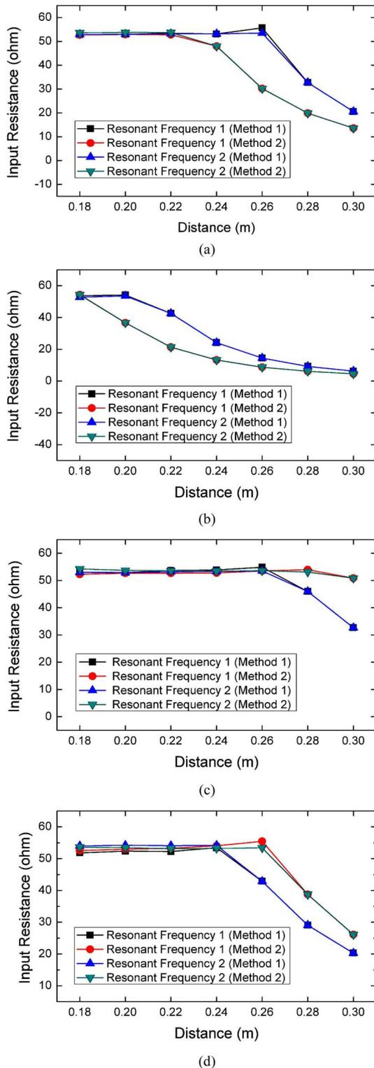
Fig. 4. Comparison of the input resistance at the resonant frequencies for two coupled small helix antennas: (a) parallel configuration, (b) diagonal configuration, (c) collinear configuration, and (d)  $\pi/4$ -tilted collinear configuration. (Method 1: the full EM simulation; Method 2: the proposed method based on the addition theorem).
