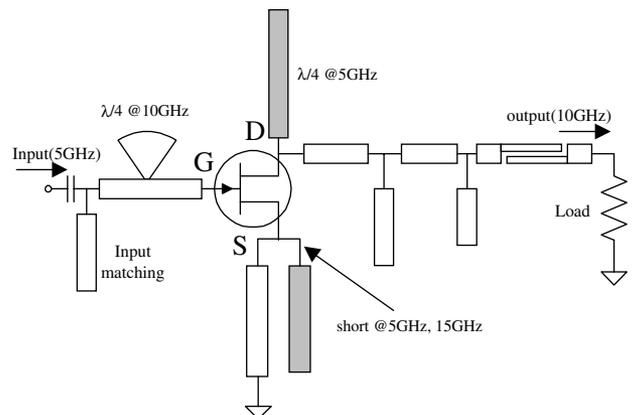
Figure 3 Schematic of the 10 GHz output frequency doubler
