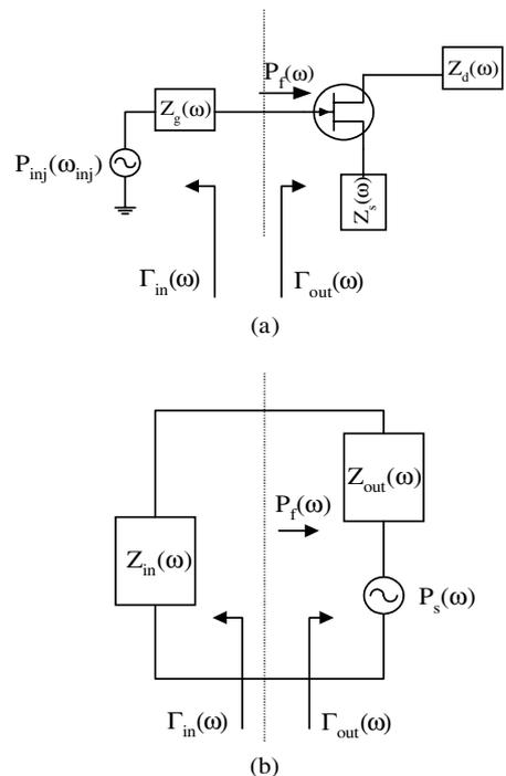
**Figure 2** ILO block diagram. (a) Three-port ILO. (b) Two-port equivalent circuit with fictitious internal source
