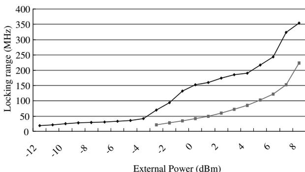
**Figure 4** Locking ranges of ILOs (frequency doublers). –■– Frequency doubler which has 5 dBm feedback signal without harmonic terminations. –◆– Frequency doubler which has 1 dBm feedback signal with harmonic terminations
