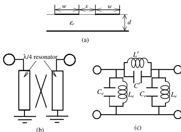
**Figure 1** Coupled microstrip-line resonator. (a) Cross section. (b)  $\lambda/4$  resonator. (c) Equivalent circuit of  $\lambda/4$  resonator
