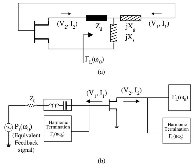
**Figure 1** Impedance substitute method. (a) Series feedback oscillator topology. (b) Equivalent circuit of the oscillator in terms of amplifier topology
