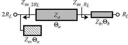
Fig. 1. Asymmetric impedance transformer, MCCT.
