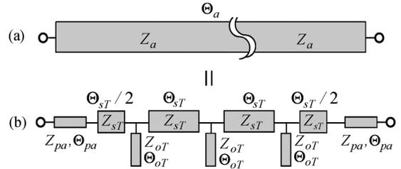
Fig. 4. SMT with  $N = 3$  (Stepped-impedance modified  $T$ -type).
