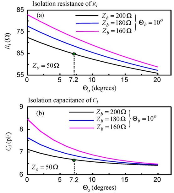
Fig. 3. Isolation Circuits. (a) Resistance. (b) Capacitance.
