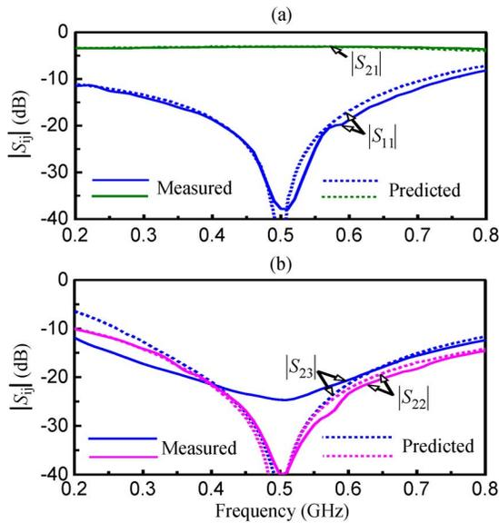
Fig. 6. The results measured and predicted are compared. (a) Power division and matching at port 1; (b) Isolation and matching at port 2.
