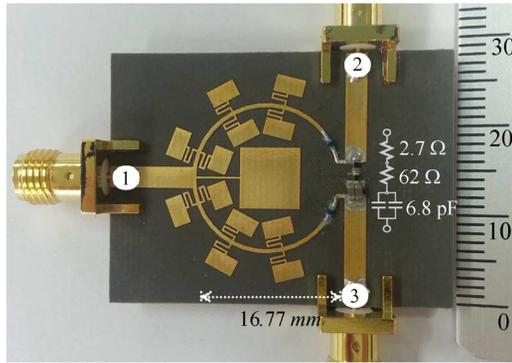
Fig. 5. Fabricated MCCT PD.
