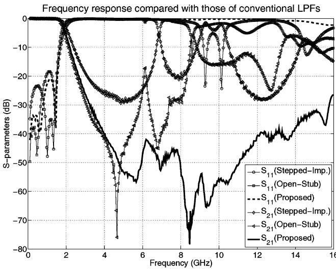
Fig. 4. Measured  $S$ -parameters of the designed LPF and conventional ones.
