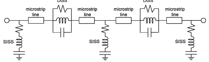
Fig. 2. Modified equivalent circuit for estimating the whole-band characteristics.
