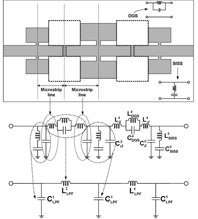
Fig. 1. Equivalent circuits for designing an LPF. (Equivalent circuits of DGSs, SISSs, and short microstrip line sections, and grouping scheme for relating them to the  $L$  and  $C$  values obtained from a prototype filter.)
