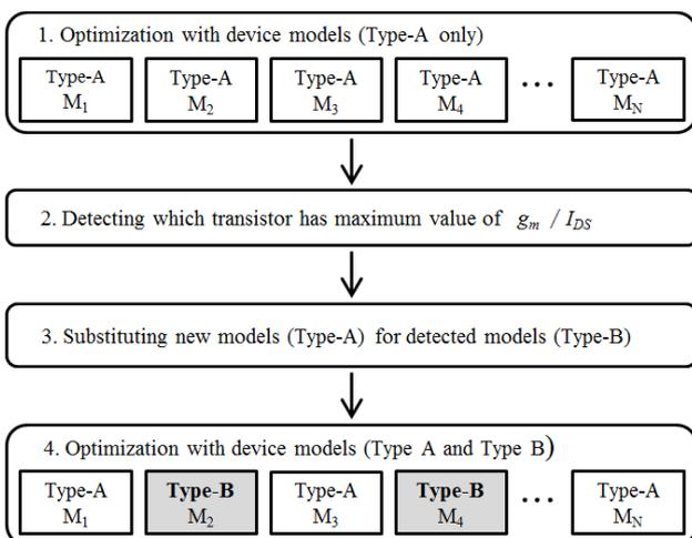
Fig. 2 Subthreshold device selection algorithm.
