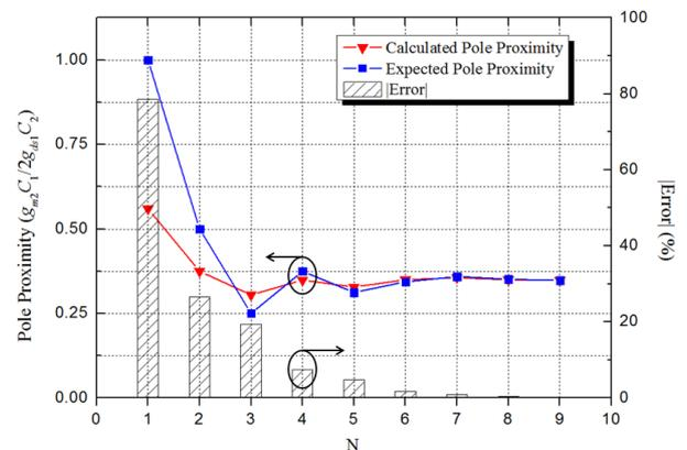
**Fig. 4** Expected pole proximity and calculated pole proximity from optimization according to the number of iterations  $N$  through the bisection method and the absolute value of the error.
