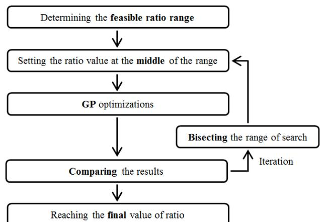
Fig. 3 Iterative optimization flow through bisection method.
