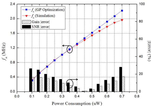
**Fig. 6**  $f_n$  versus power consumption from the GP optimization and the simulation and absolute value of the error between the GP and the simulation for gain and SNR.
