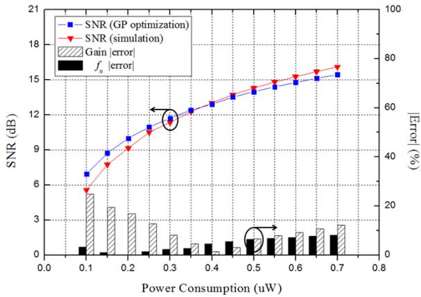
**Fig. 5** SNR versus power consumption from GP optimization and the simulation and absolute value of the error between GP and the simulation for gain and  $f_n$ .
