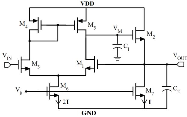
Fig. 1 Second-order active filter schematic.
