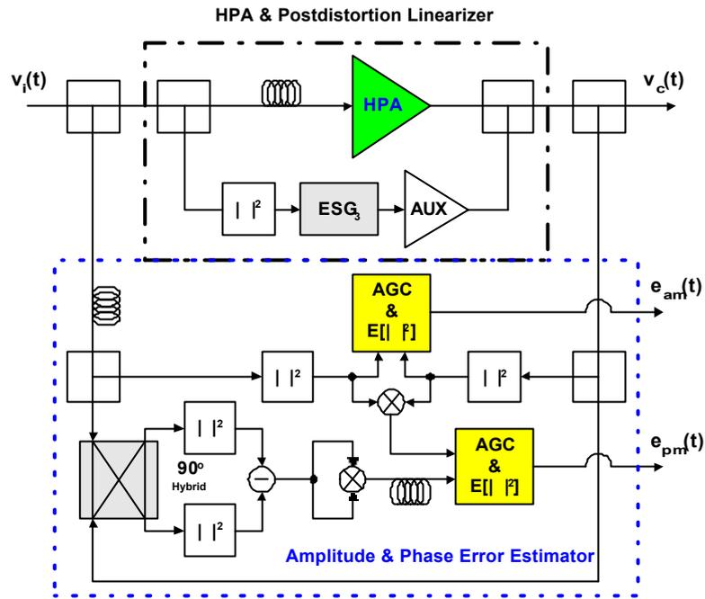
Figure 1: Block diagram of the proposed estimator
