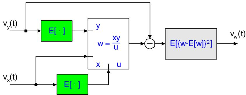
Figure 2: Block diagram of the AGC and averaging circuit
