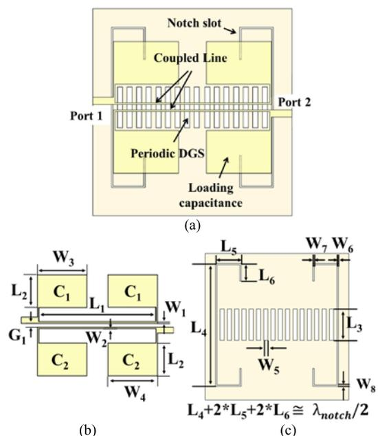
**Fig. 1** The proposed DC block. (a) Overall-view, (b) top-view, and (c) bottom-view.
