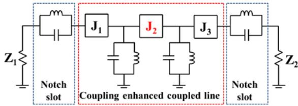
Fig. 2 The equivalent circuit of the proposed DC block.
