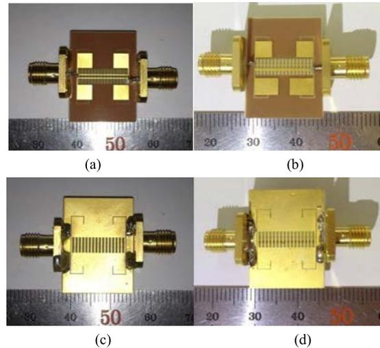
Fig. 3 The fabricated DC blocks. (a), (c) : 50 and 50  $\Omega$  terminated DC block top and bottom view. (b), (d) : 50 and 30  $\Omega$  terminated DC block top and bottom view.
