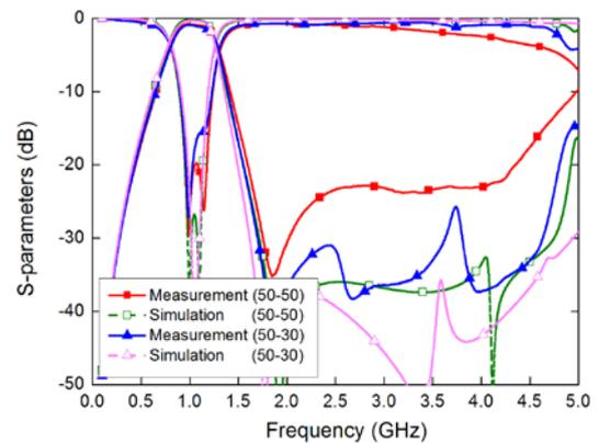
Fig. 4 The simulation and measurement results: 50 and 50  $\Omega$  terminated DC block and 50 and 30  $\Omega$  terminated DC block.
