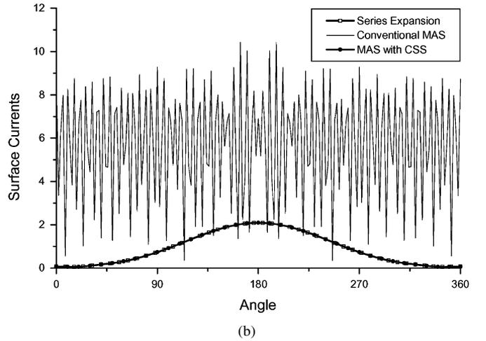
Fig. 3. Surface currents calculated from series expansion, conventional MAS, and MAS incorporating CSS for the case of (a)  $k_0R = 2.4048$  and (b)  $k_0R = 2.8292$ .
