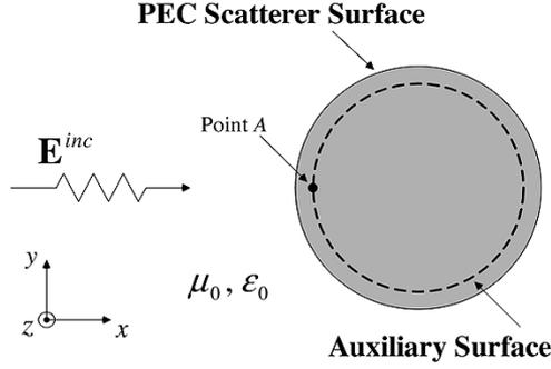
Fig. 2. 2-D circular cylinder illuminated by a TM-z polarized plane wave.
