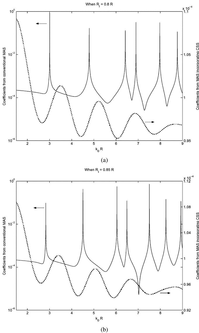
Fig. 4. Absolute values of the coefficients of the AS at point A in Fig. 2 calculated from conventional MAS (log scale, solid line) and MAS incorporating CSS (linear scale, dotted line) for the case of (a)  $R_i = 0.8R$  and (b)  $R_i = 0.85R$ .
