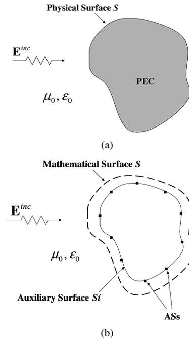
Fig. 1. (a) PEC scatterer illuminated by an incident wave. (b) MAS model equivalent to the situation in Fig. 1(a).
