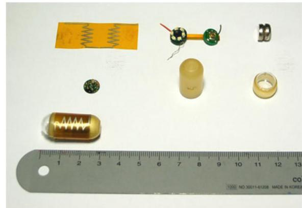
Fig. 9. Photo of the integrated capsule endoscopy with outer antenna.
