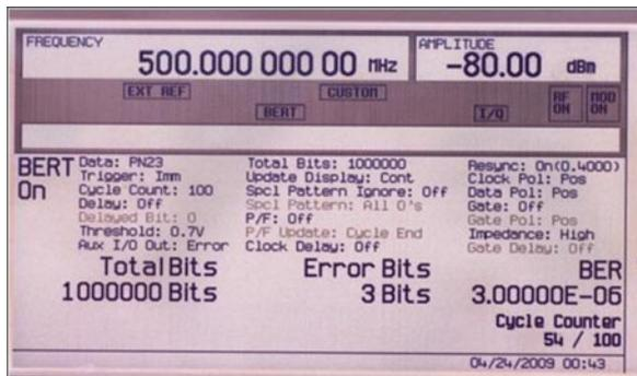
Fig. 8. Bit-Error-Rate test results at Agilent E4438C.
