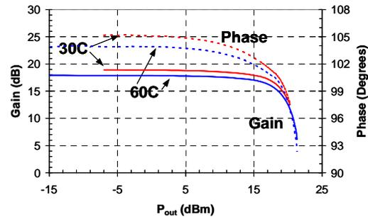
Fig.6: Measured variation of gain and phase with output power at several temperatures
