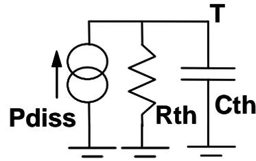
Fig. 7: The equivalent thermal circuit
