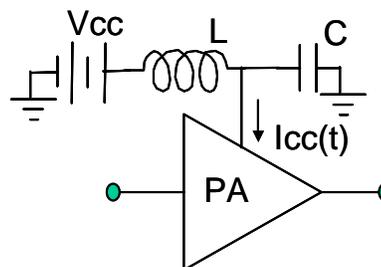
Fig.4: Schematic diagram showing bias circuit
