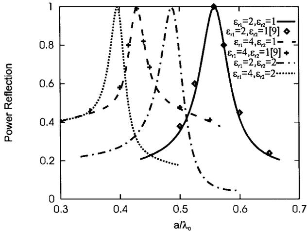
Fig. 1. Power reflection coefficient of a crossed-dipole FSS sandwiched between two dielectric substrates.
