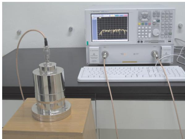
Figure 4 Set up of EMSE testing apparatus.
