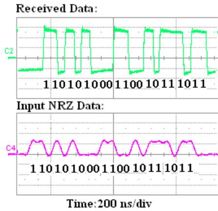
Fig. 8 Measured input and output waveforms for the data rate of 40 Mbps
