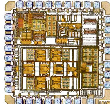
Fig. 7 Chip microphotograph of the OOK receiver
