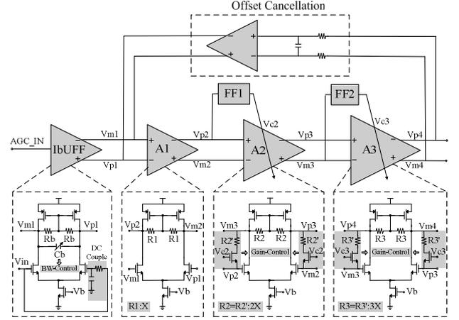
Fig. 6 Discrete-step AGC with offset cancellation
