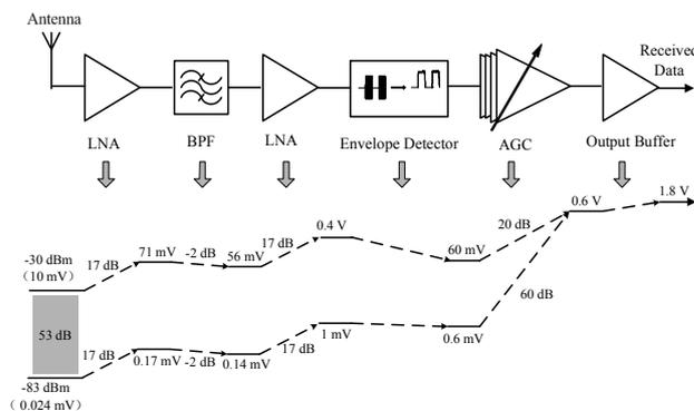
Fig. 1 OOK receiver architecture and power strength level flow
