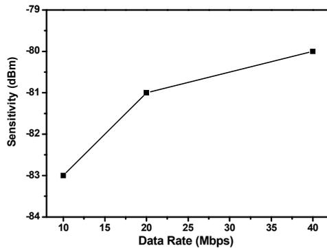
Fig.9 Measured sensitivity summary of the OOK receiver
