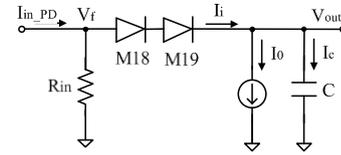
Fig. 4 Simple equivalent structure of peak detector
