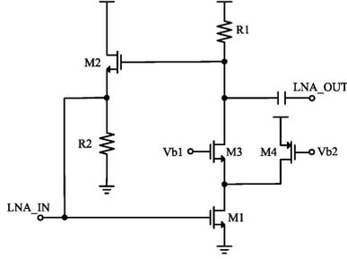
Fig. 2 Schematic of the single-ended LNA
