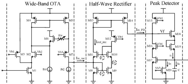
Fig. 3 Schematic of the proposed envelope detector
