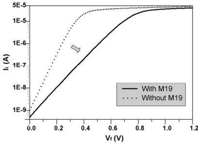
Fig. 5 I-V characteristics with and without M19, respectively
